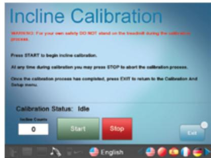
5. Select Incline Calibration on the Calibration and Setup screen.
