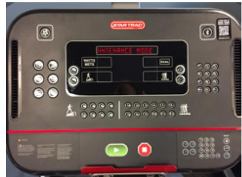
3. Press the **↓** until the marquee window reads "MODEL". Verify that the model shown on the right side of the information window matches the base it is installed on (i.e. 8TR vs 8TRx).
